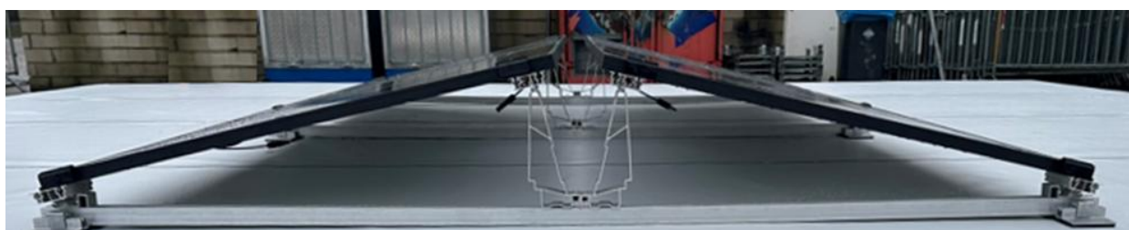
Figure 4 – Side view of the East/West-orientated PV array.
