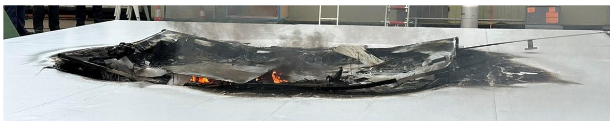
Figure 13 – From the end of test 1, where the EPS was initially ignited and subsequently melted below the PV array. The closest PV modules are PV4 (left) and PV2 (right) in accordance with Figure 5.
